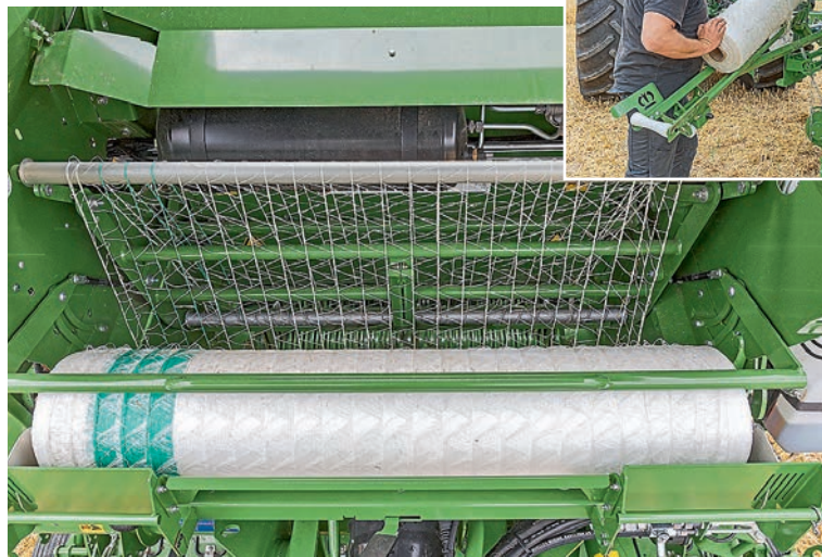
Threading the net is relatively straightforward, and the pivoting side chute makes loading a fresh roll a lot easier.
