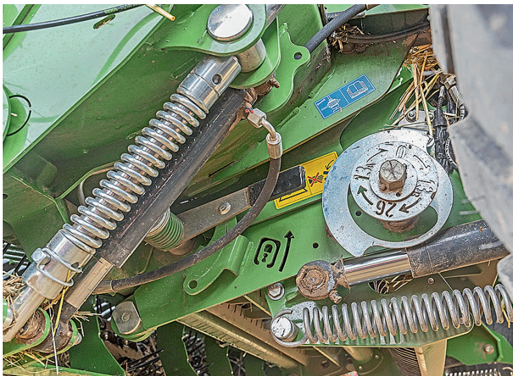
The knife release and the hydraulic control are located on the left-hand side.
