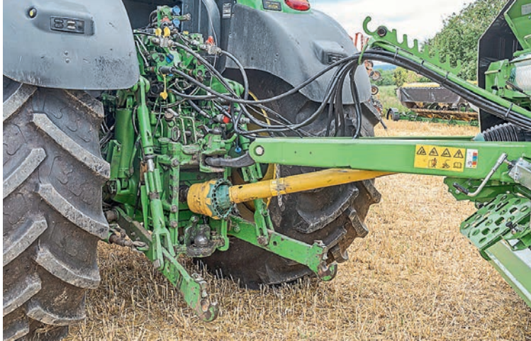
Shown here in its upper position, the drawbar can be adjusted for use with a lower hitch mounting. The hoses and cables are tidily routed through the rack.
