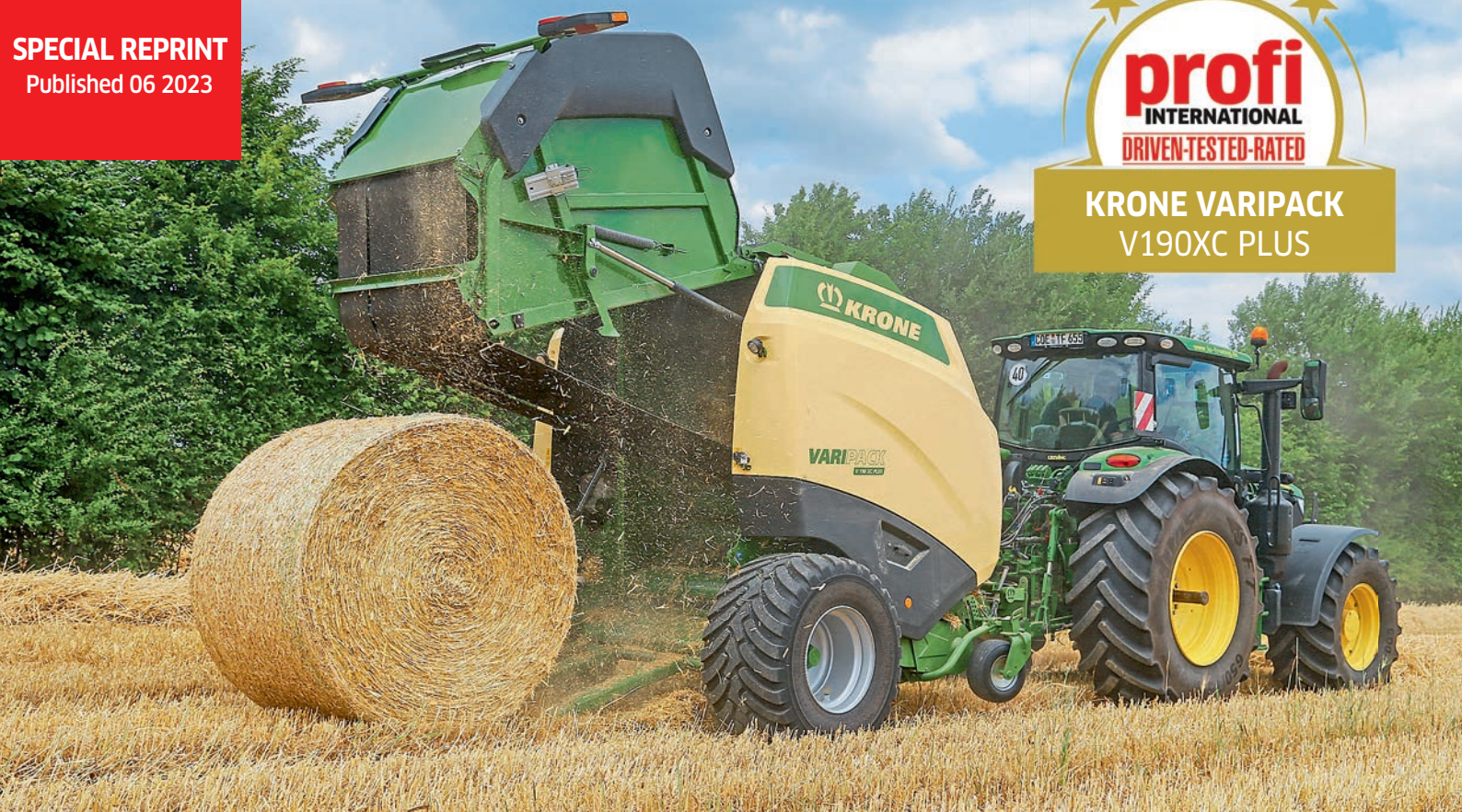
Straw was the main crop we tackled with the VariPack V190XC Plus variable-chamber belt baler in our practical test.
