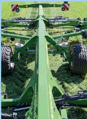
New trapezoidal central beam is designed to prevent vibrations and improve the stress load distribution on the machine.
