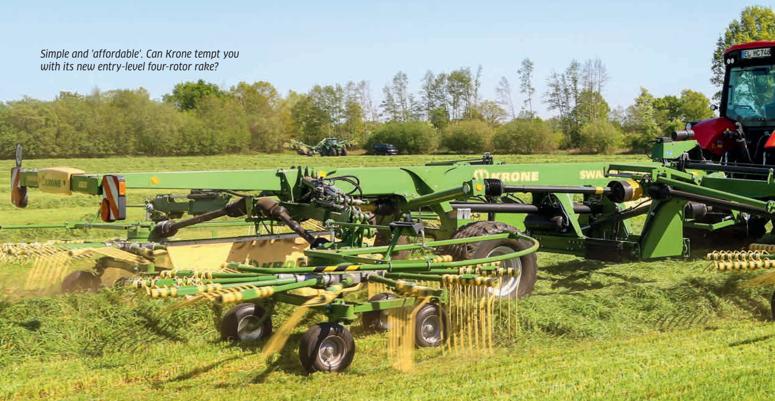
New trapezoidal central beam is designed to prevent vibrations and improve the stress load distribution on the machine.
