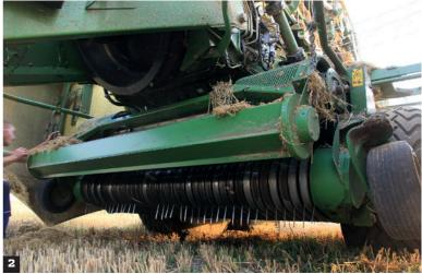
only half the knives are in action, they cut the crop to lengths of 88 mm; when no knives are selected, the machine obviously doesn't cut at all. The feed tines are arranged in a V and are Hardox plated for a long service life.
