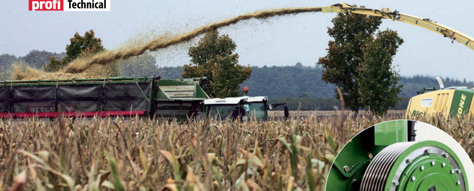
Krone now offers a gearbox for the chopping drum on its BiG X 600 to 1100 series models – the VariLOC.
