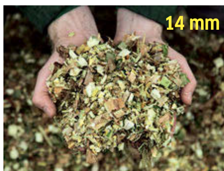
The quality of chop obtained in our test on a BiG X 700 with a 36-blade MaxFlow chopping drum, a VariLOC gearbox and a disc cracker can be seen here. The nominal LOC was set to 4mm (left), 14mm (middle) and 24mm (right). The kernels were effectively crushed in all samples. Photos: Eikel, manufacturer (1)
