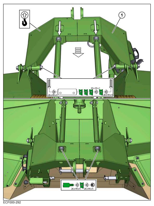
4.19 Mounting the three-point hitch ("Pushed three-point hitch" version)
