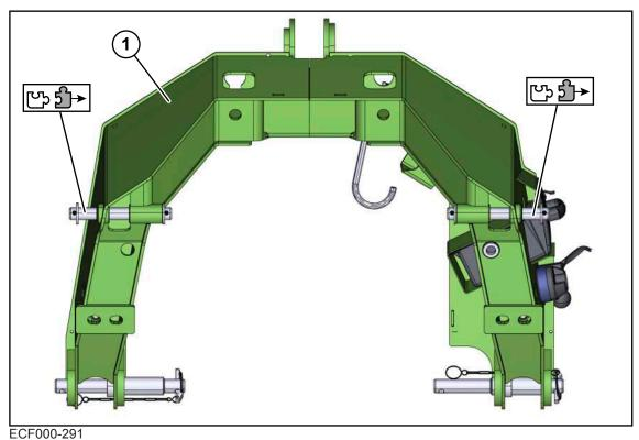
Mounting the three-point hitch ("Pushed three-point hitch" version) 4.19
