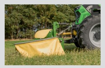
A clean cutterbar The sloping deck and the stretched curtains prevent ingress of debris and the cutterbar stays clean.
