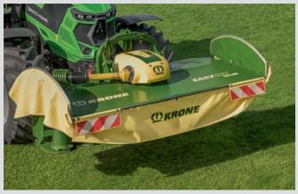
**Compact on the road** Although offering a 3.16 m cutting width, the EasyCut F 320 M and F 320 fold into a very compact transport unit. The ends of the curtain guard fold back to bring the transport width down to 3.00 m. A hydraulic fold mechanism is an option.
