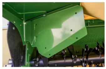
Adjustable swath width The standard swathing plates swath the material to any width and infinitely variably. The plates are stored on the machine when not needed.
