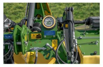
**Best adaptation to the ground** The hydraulic mower suspension and the new headstock provide more than 1 m up/down travel and perfect contouring.
