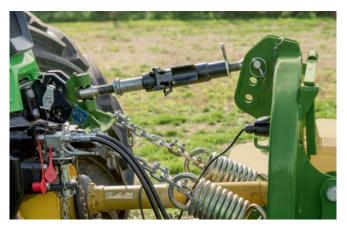
**Contouring in direction of travel** The flexible and telescoping top link (option) allows the mower to follow any contour and produce a perfect cut.
