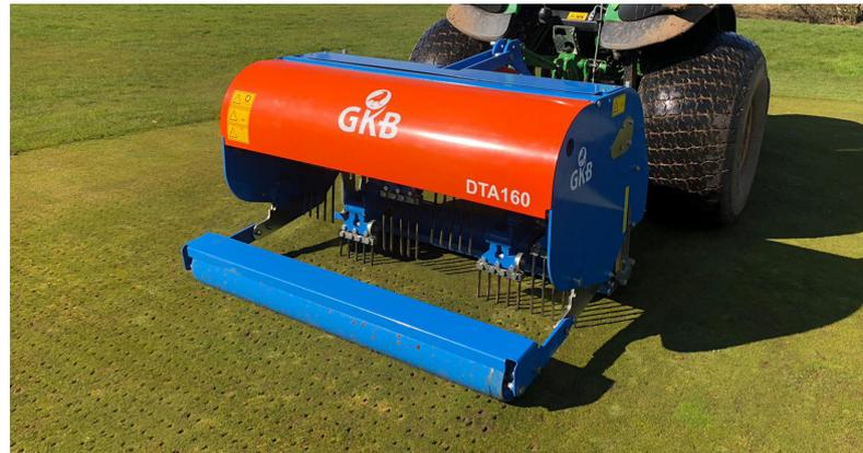
With an adjustable 25-degree heave angle, the Deep Tine Aerator's tine holding system allows you to take control on removing compaction from various depths up to 40 cm.
