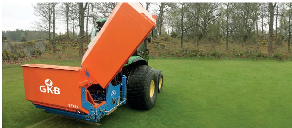
As the foundation of the Sandfiller we are making use of the clarified principle of the much-praised Combinator. The slitting rotor is provided with an attachment to the carbide blades that create wind to move the material to the sideways-tipping container. After you have emptied the sideways-tipping container, you can simply refill the container with dried sand.
